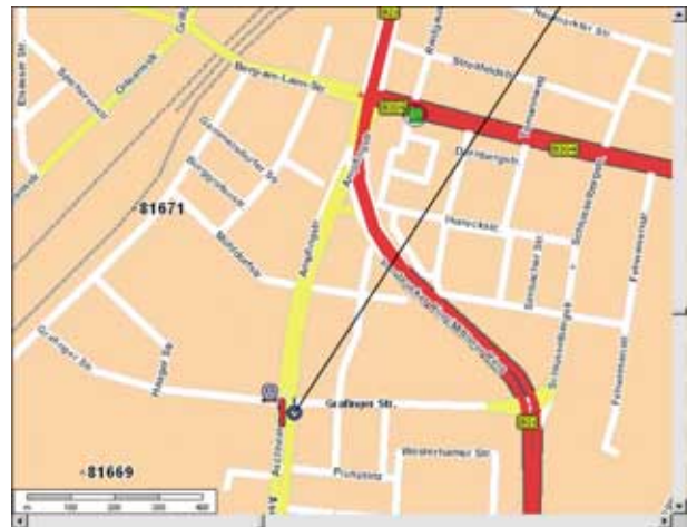
Fig. 2: Display in a homing DF system. On the left-hand side of the DF symbol is the receive level display. The system can be conveniently operated without using a keyboard; all menus that are not required during driving are deactivated.
